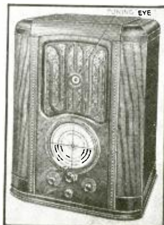
Fig. B. An "export" and "marine" set such as described by the author. This set is designed to withstand unusual climatic and temperature changes as well as shipment in "freighters."
