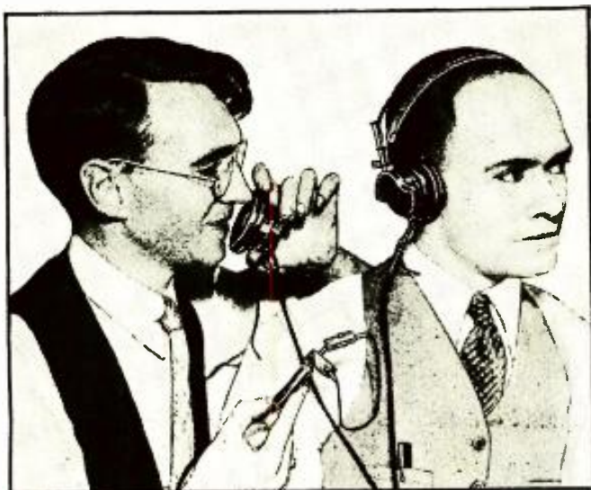
Fig. A. A "trick" to illustrate dynamic-type phones used as transducers. Whispering into one phone can be heard with good volume in the other.
